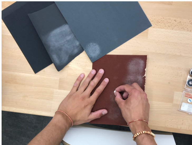
Figure 18: The process of polishing the surfaces of the model retinas with sandpaper of different grain sizes
