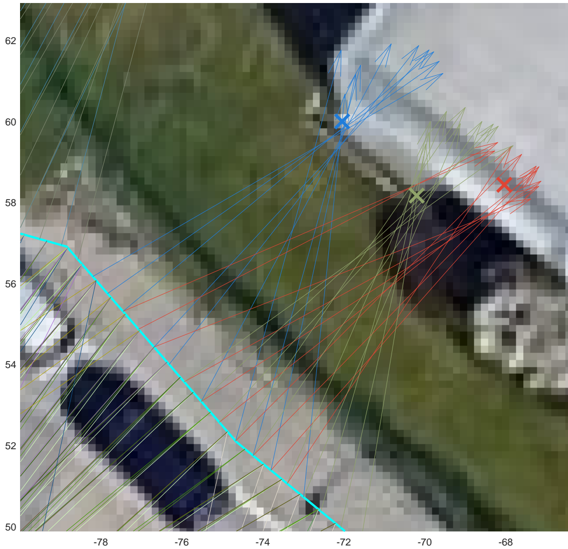
Figure 6.10: Urban landmark localized from the sequence of images in Figure 6.8 – blue arrows point from the place of image acquisition in the extracted direction of the landmark. Blue cross represents the triangulated location of the landmark in the map. Similarly, red-colored markers belong to landmarks shown in 6.9 with the two mis-identified landmarks aiming more to the left. Other colors denote yet another landmarks.
