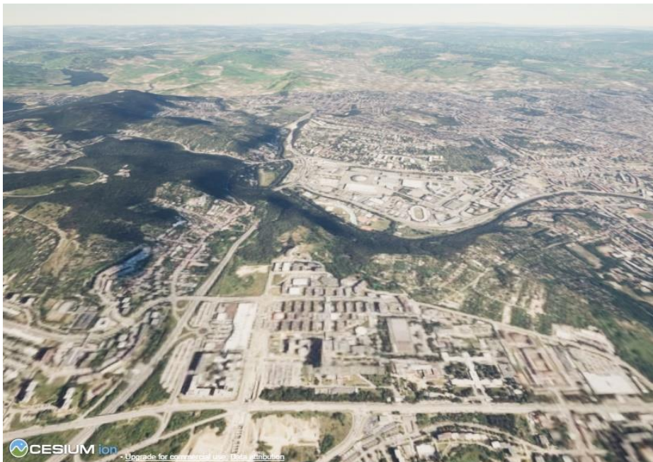
Figure 9: Unreal Engine 4 running the Cesium for Unreal plugin. The scene depicts a combined elevation and imagery layer for Brno. The Cesium Ion watermark is visible since the content is streamed from this platform without a commercial license.
