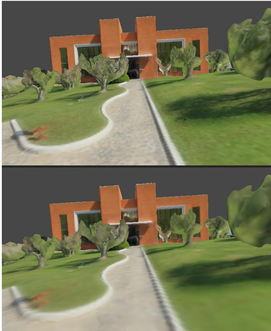
Figure 10: Comparison of two pictures showing a part of ESRIN within Unity at different texture resolutions (top: 8192x4, bottom 4096x4). The reduction by a factor of four leaves bricks, leaves, and grass completely smoothed and reduced the file size for each individual texture from 256MB to 64MB.
