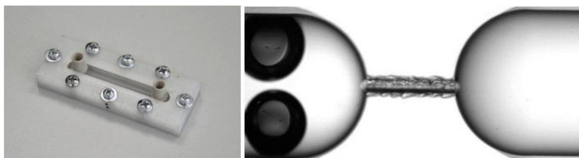
Obr. 3.1 – Sestava čipu a detail clonky [25]
