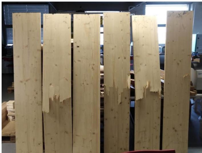
*Figure 21 – Tested thin plate samples*
