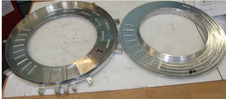
Fig. 2-1 Segments of the cooling jacket eventually creating the duct in the middle after assembly
