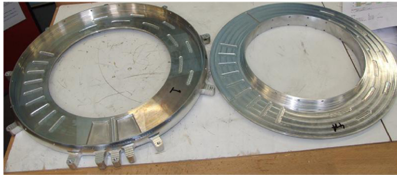
Fig. 2-1 Segments of the cooling jacket eventually creating the duct in the middle after assembly
