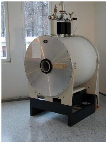
Obr. 36: MR tomograf Bruker Biospec 4.7 T [9]
