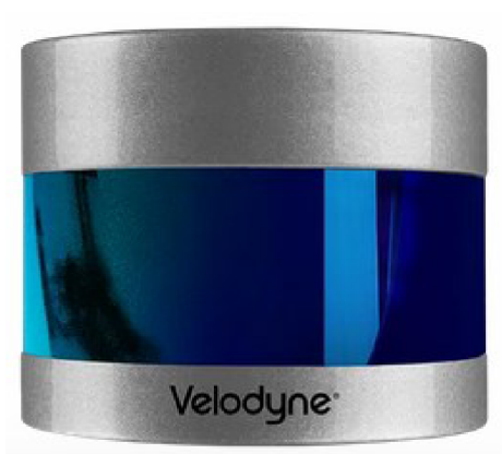
Obr. 8 Velodyne Ultra Puck surround LIDAR [18]
