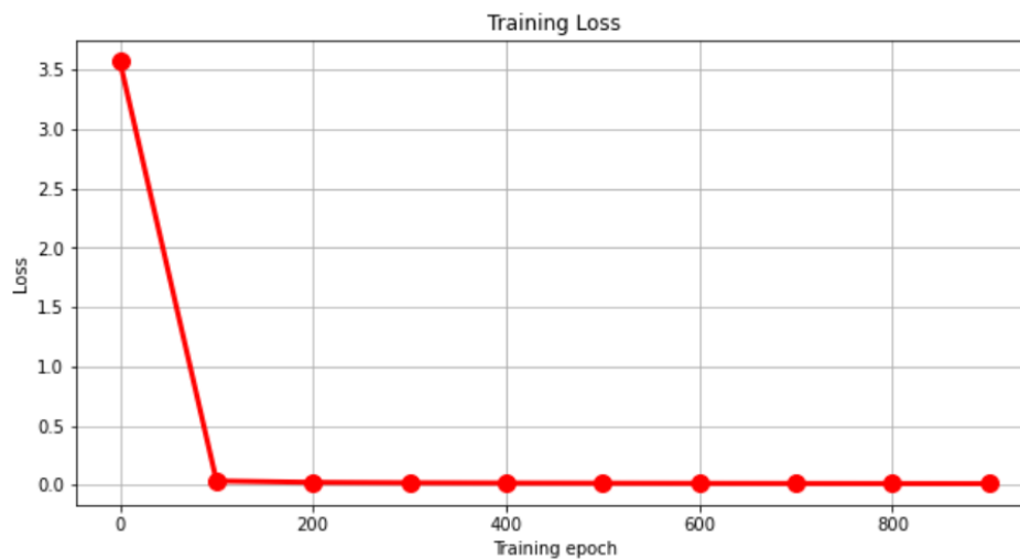
Figure 5.11: The Training Loss of Network Layer IDS at each layer (epoch). Own Visualization.
