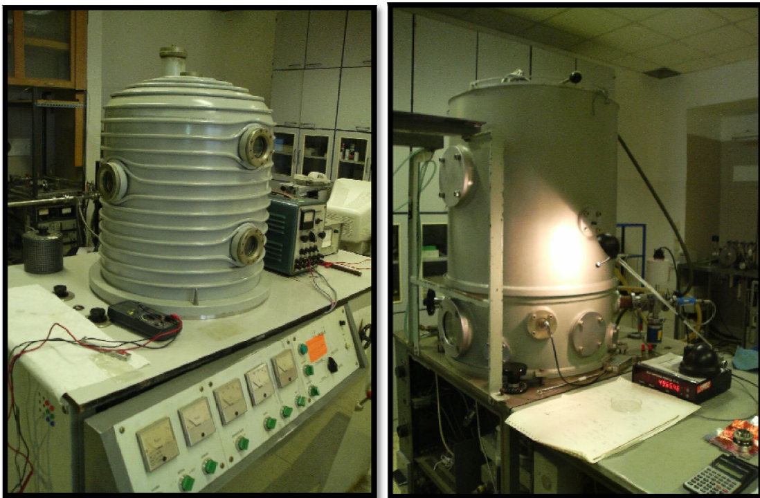
Picture 9 - Vapour depositors
