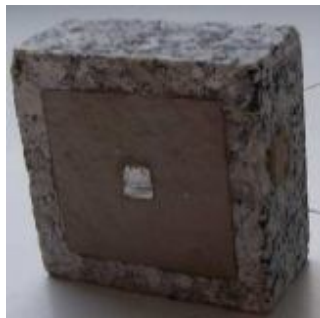
Fig. 5.60: The rock sample of granite. There is electric contact on the sample fixed by DiAg paste
