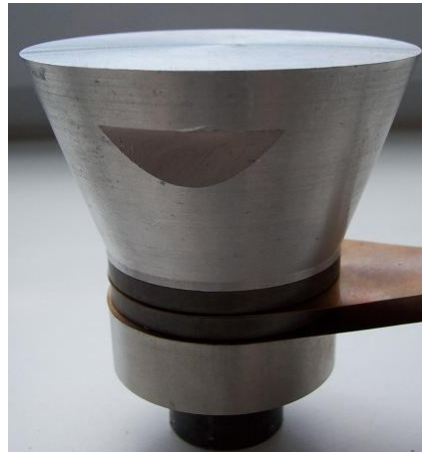
Fig. 4.8: Ultrasonic actuator with cylindrical body which has radius 80 mm denoted HTP02
