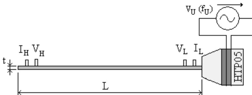
Fig. 5.20: The sample of the Mg alloy flat cross-beam fixed on the ultrasonic actuator, I_L , I_H , and V_L , V_H are current and voltage contacts, respectively.
