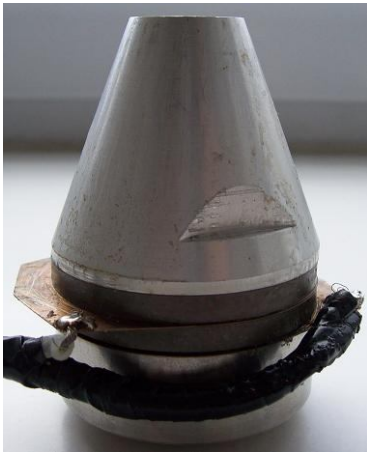
Fig. 4.7: Ultrasonic actuator with cylindrical body which has radius 20 mm denoted HTP 05
