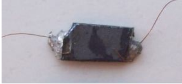
Fig. 5.35: Specimen of monocrystal CdTe
