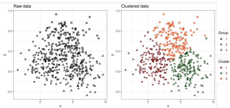
FIGURE 2.5: Left panel show randomly generated data-set drawn from multivariate normal distribution consisting of three groups (denoted by shapes); Right panel shows the same data-set clustered using K-means algorithm (clusters are highlighted using various colours)
