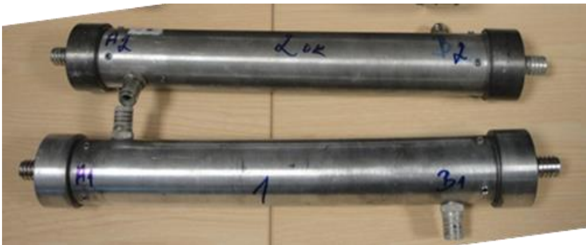
Fig. 35 PHFHE-1 and PHFHE-2 in stainless steel shell
