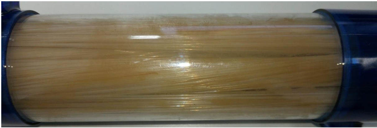
Fig. 28 External view of PA-72 PHFHE after tests
