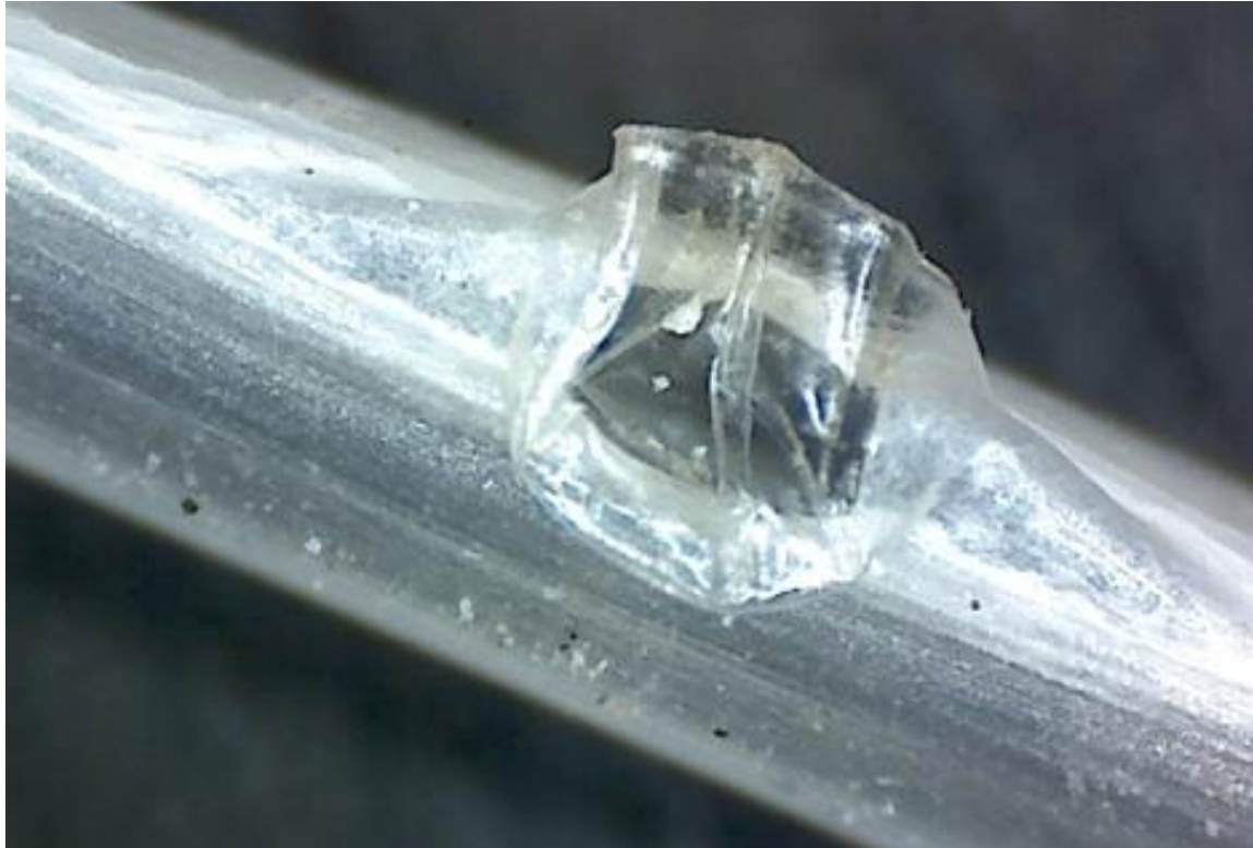
Fig. 14 The defect of PP-RCT fiber occurred at the temperature 80°C and the pressure 40 bar
