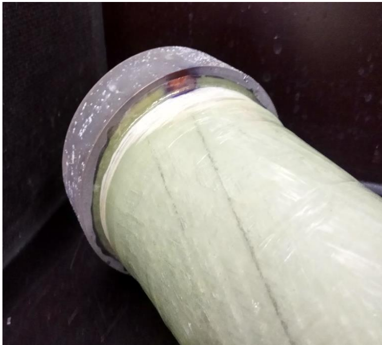
Fig. 53 Leak location in PHFHE Wind-1 after static pressure tests
