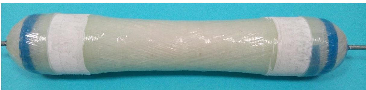
Fig. 46 External view of the PHFHE at the end of the second creation stage
