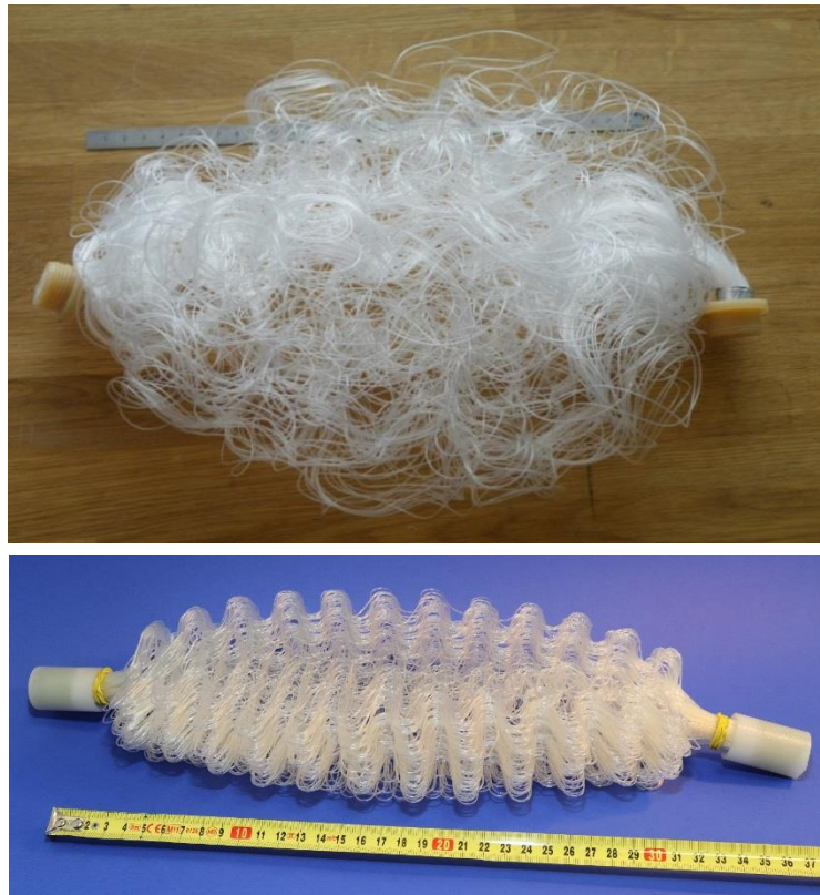
Fig. 15 Overall view of polymeric hollow fiber bundle with chaotic (top) and semi-chaotic (bottom) structure
