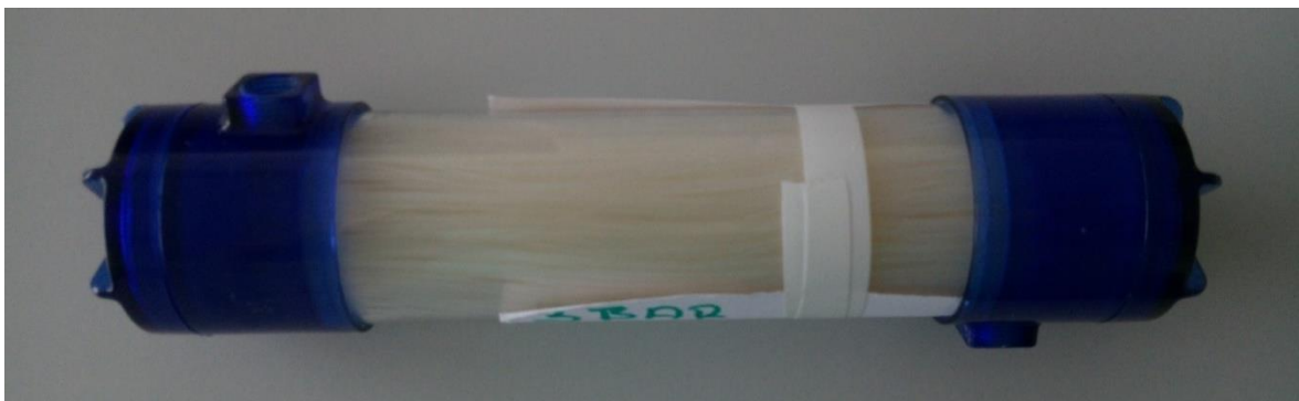
Fig. 23 Overall view of PA-72 PHFHE
