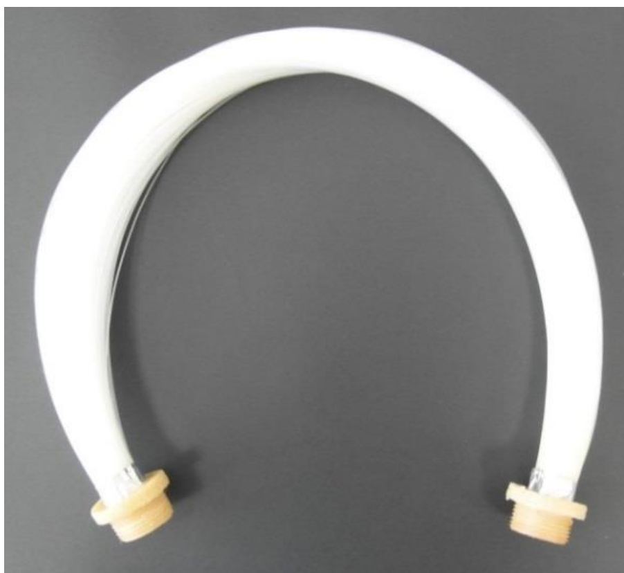
Fig. 13 Overall view of a PHFHE with a straight hollow fiber bundle
