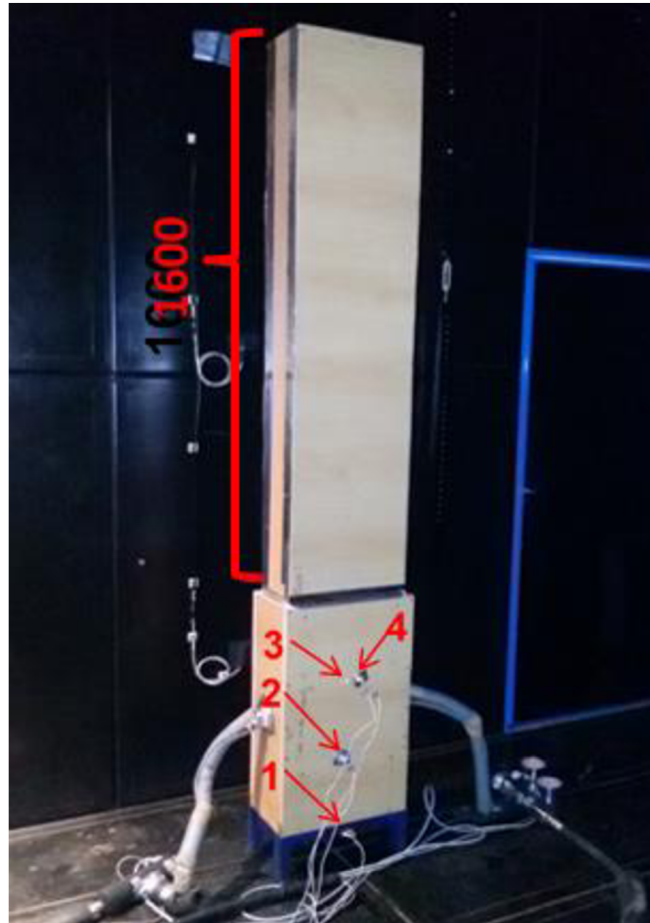
Fig. 22 Overall view of the heat exchanger with one hollow fiber bundle and a tube.
