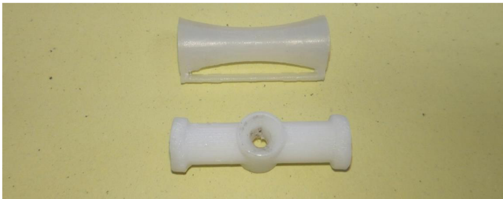
Fig. 41 Improved feeding heads
