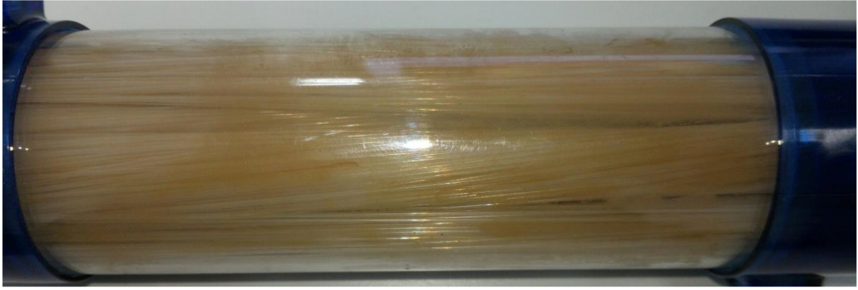
Fig. 28 External view of PA-72 PHFHE after tests
