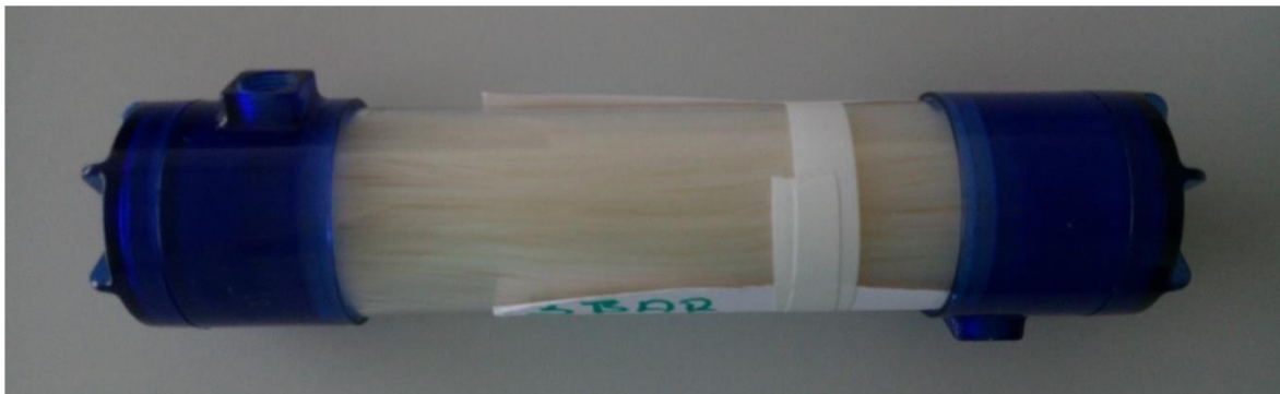
Fig. 23 Overall view of PA-72 PHFHE
