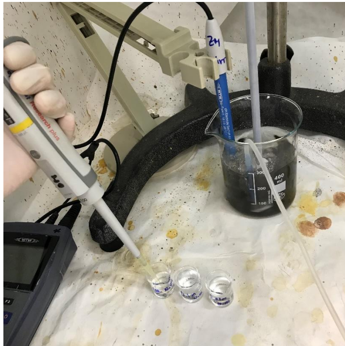
Figure 10 Adjusting of pH via dosing of NaOH from beakers containing (0.01M, 0.1M or 1M) (Porter 2019)
