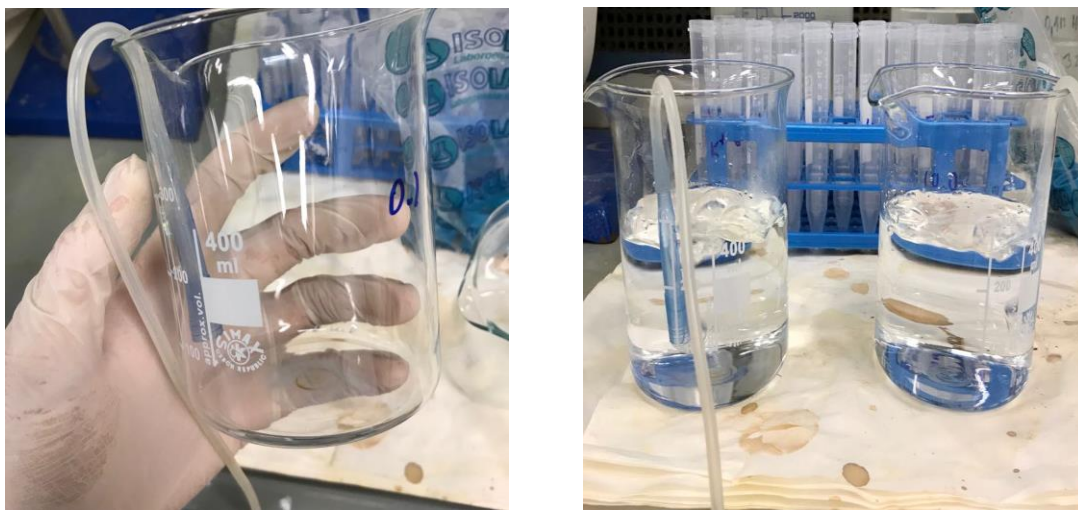
Figure 7 Apparatus for introduction of nitrogen atmosphere (left), Gas sparging the metal solutions until all additional gasses are sparged (right) (Porter 2019)
