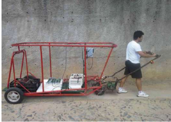
Figure 3.6: Mechanical traction system for electrical load cart developed by L. A. Silva et al [27]
