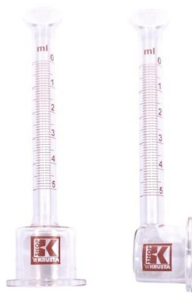
Figure 12 Karsten testing tube, left for horizontal surfaces, right for vertical surfaces measurement
