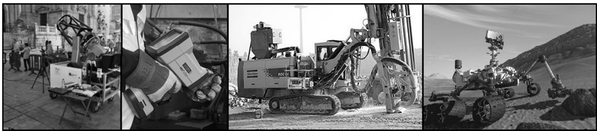
Figure 4 , advanced LIBS devices (from left to right): stand-off LIBS system during the measurement of the facade of the historical building in Malaga, Spain (the group of Javier Lasserna); handheld LIBS (Lasersec Systems) for direct analysis; LIBS device attached directly to the mining machine (the group of Reinhard Noll); ChamCam LIBS system attached to the Mars Rover, Curiosity.
