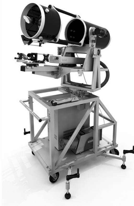
Figure 1 , schematic diagram of the stand-off LIBS device.
