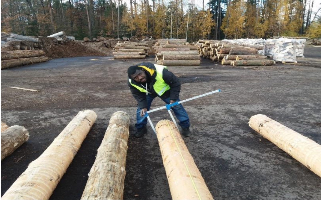
Figure 15. Diameter measurement of small end of a spruce log with a calliper
