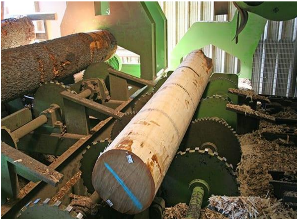
Figure 8. Log debarking machine debarking log
