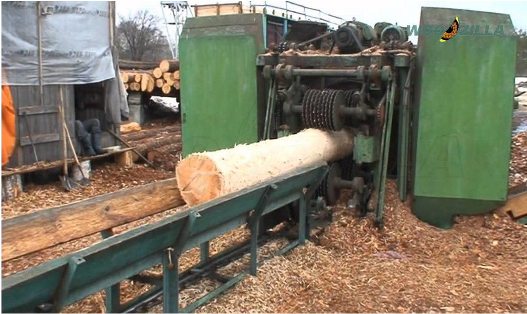
Figure 7. Log debarking machine debarking spruce log
