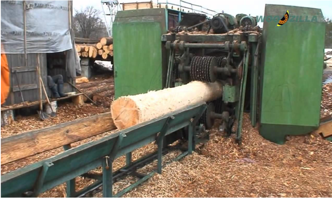
Figure 7. Log debarking machine debarking spruce log
