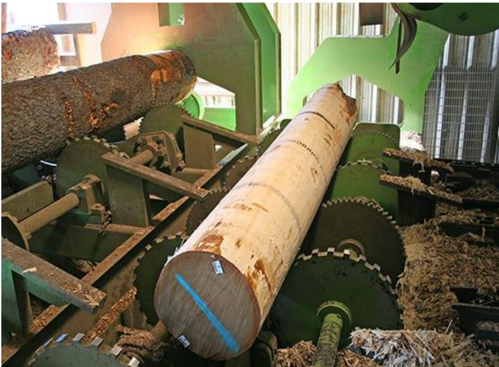
Figure 8. Log debarking machine debarking log
