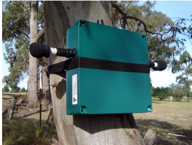
Figure 13. Song Meter SM2+ batcorder (Source: www.fivethirtyeight.com )
