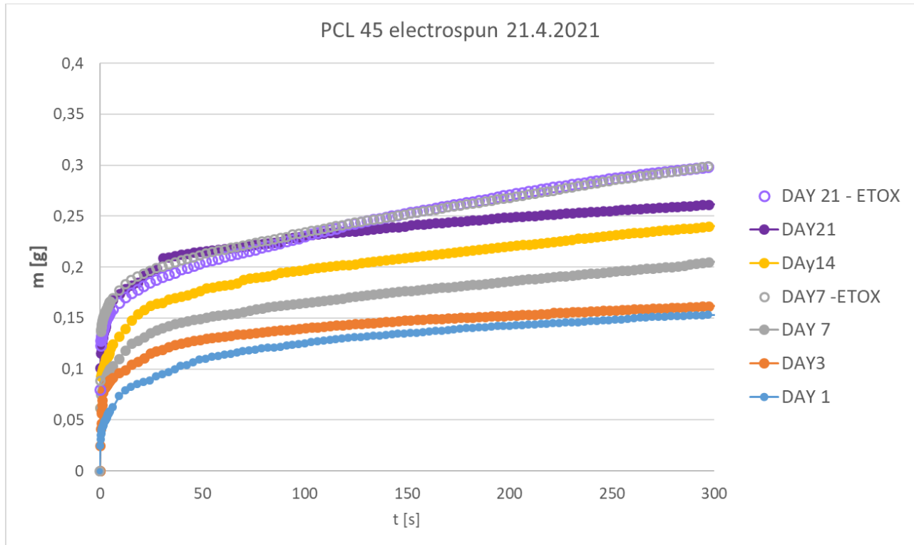
Figure 37. Graph of average data from water wicking measurement by force micro tensiometer Krüss K100 for PCL-45 electrospun in April 2021 with normal sample and Ethelene oxide treated for sterilization (each single line is the average of 10 reading)
