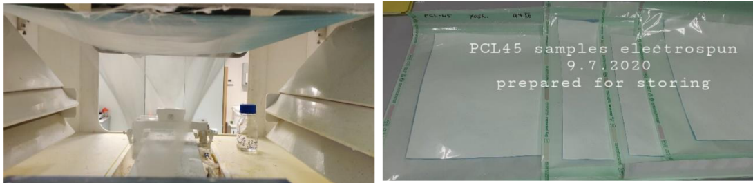
Figure 25. Electrospinning of PCL and sample preparation for storage
