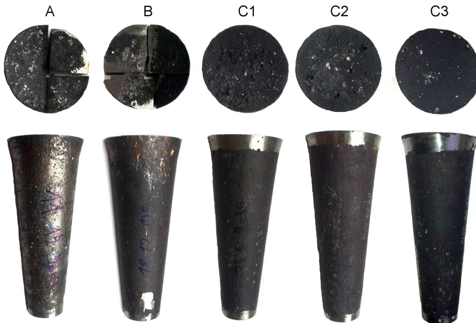
Fig. 3.2: The cone shaped ingots of 30 (bottom) and 70 (top) mm in diameter and 180 mm in length. The ingot melting route is given using capital letters.
