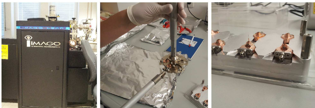
Fig. 2.7: IMAGO LEAP microscope and AP needle-shaped samples.
