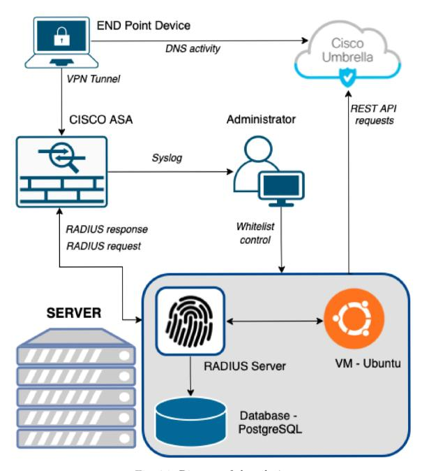
Fig. 4.1: Diagram of the solution
