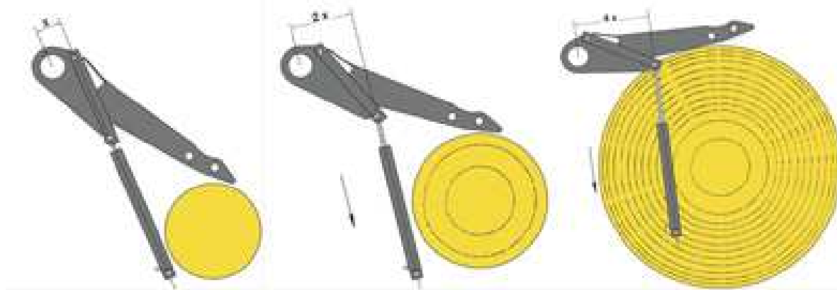
Obr. 22: Systém PROGRESSIVE DENSITY lisu Vicon
