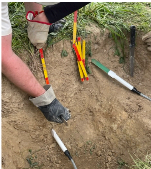
Fig. 22: Metal tool being placed into the soil profile with the flat segment perpendicular to the upper edge of the soil pit
