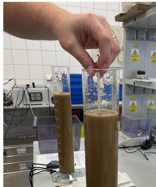
Fig. 19: The stabilization of the hydrometer prior to the measurement of solution density
