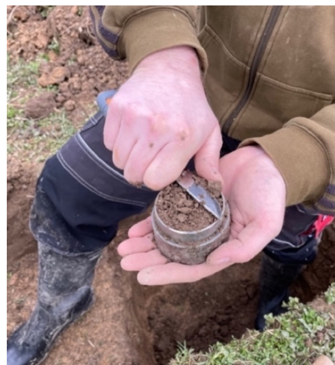
Fig. 15: Trimming of the soil sample until level with the edge of the sampling cylinder
