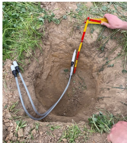
Fig. 23: Installed 25 cm and 50 cm TMS monitors
