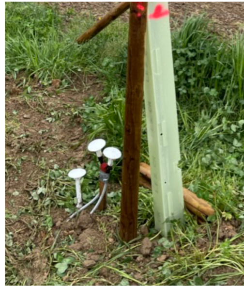
Fig. 25: Completed installation of the 14 cm, 25 cm, and 50 cm TMS monitors in the agroforestry alley
