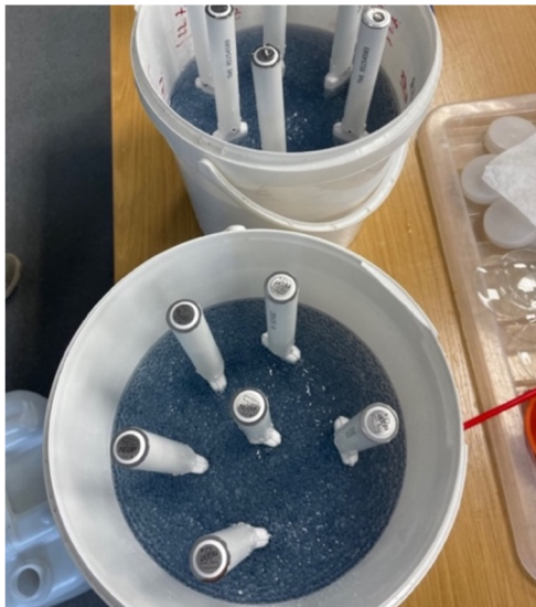
Fig. 20: TMS dataloggers placed in saturated glass marbles during the standardization process
