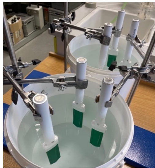
Fig. 21: TMS dataloggers placed in water during the standardization process
