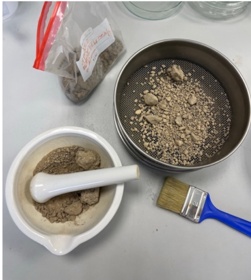
Fig. 16: Desiccated aggregates being broken down with a mortar and sieved through a mesh with a diameter of 2 mm
