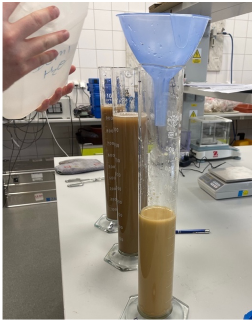
Fig. 18: Graduated cylinder containing fine soil particles being diluted to a volume of 1000ml with demineralized water
