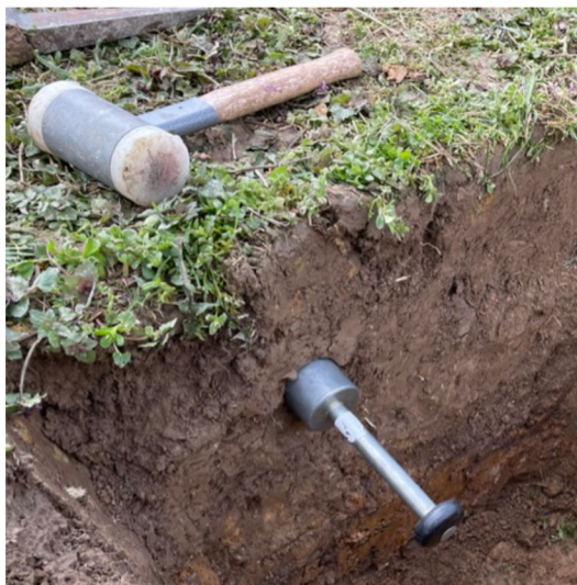
Fig. 14: Soil sampling device driven into the soil profile
