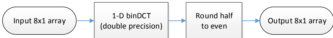
Fig. 2.2: One dimensional binDCT model flowchart
