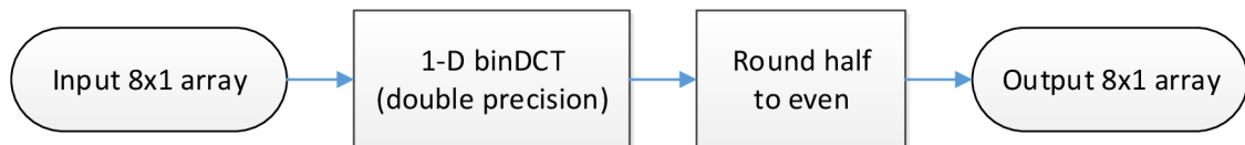
Fig. 2.2: One dimensional binDCT model flowchart
