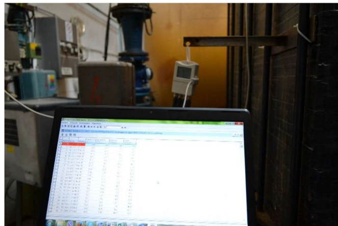
Picture 4.1. Data logger S0141 Picture 4.2. - Downloading measured data [9]
