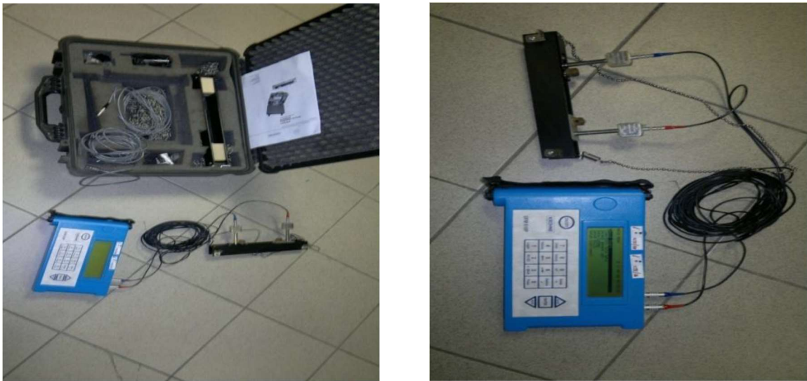
Picture 4.6. Portable ultrasonic flow meter UFM 610P Krohne [9]
