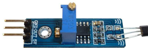
Obr. 25: Modul s Hallovou sondou A3144
