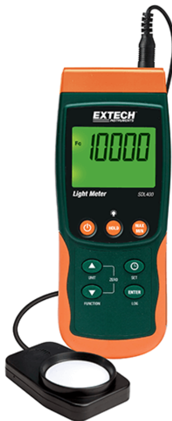
Obr. 5 – Luxmetr Extech SLD400 [24]
