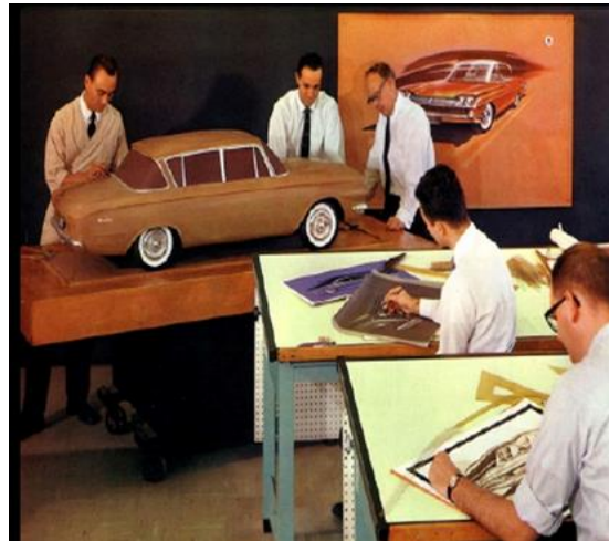
Fig 3 American motors scale model studio (1961) 1:3 clay model. [8]
