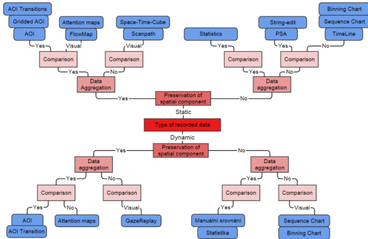
Fig. 1 Decision scheme for selection of methods for the analysis of eye-tracking data
