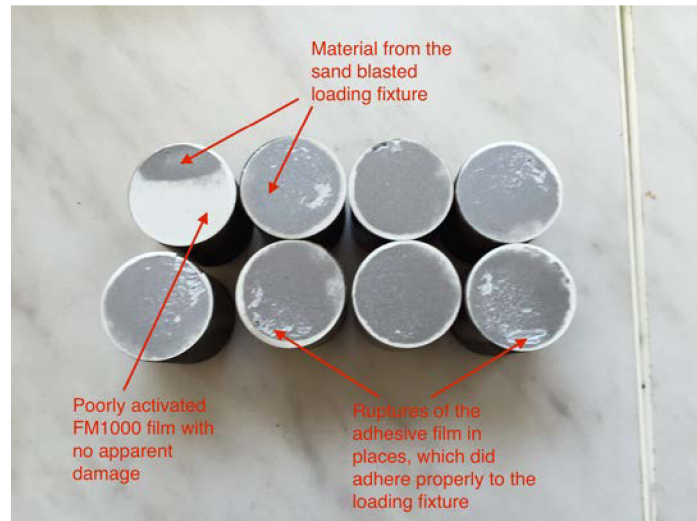
Figure 43 - Series of adhesion tests of specimen B (grinded). Failure occurred in the adhesive film
