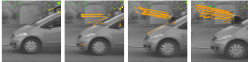
Figure 7: The 6D-Vision algorithm detecting a pedestrian behind a vehicle.[16]
