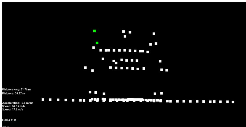
Figure 35: Object detected in LIDAR frame 0 of sequence 1 with the number of points used for detection colored in green.
