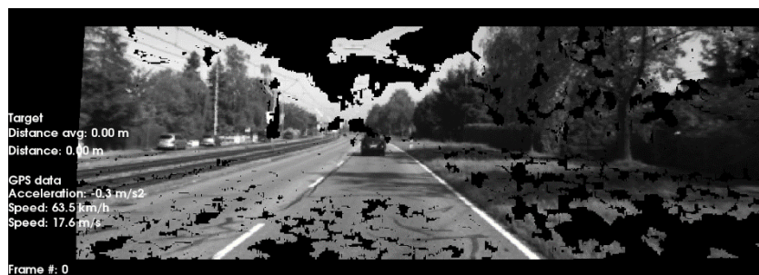
Figure 19: An example reprojection from the camera point of view. No depth information is available for the black regions because the disparity was not estimated during stereo matching.
