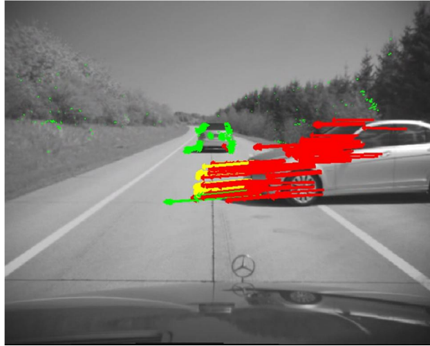
Figure 8: 6D-Vision detecting a vehicle entering the driving corridor from the right side.[16]
