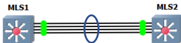
Picture 26 Etherchannel between MLS1 and MLS2
