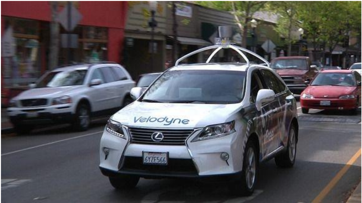
Figure 15 Car collecting data in real traffic for statistical testing
