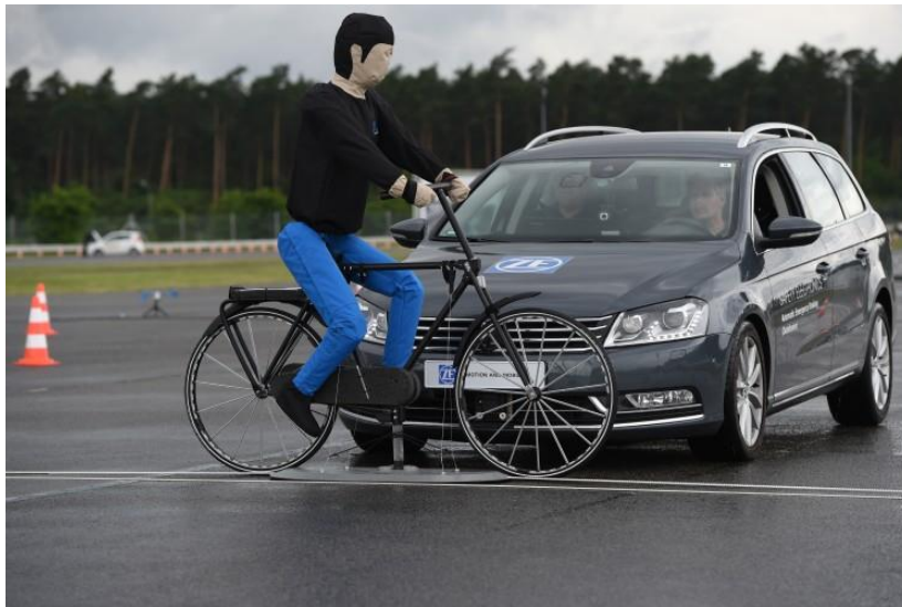
Figure 9 Predefined test of AEB for cyclist detection
