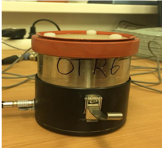
Figure 19. Transferring sample from KSAT to Hyprop unit. At the top of the sample is a porous membrane used as a mechanical support by the Ksat device.
