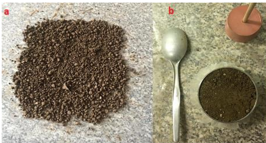
Figure 14. Control sample was left to air dry after spraying water (a) and repacked into Kopecky ring (b).
