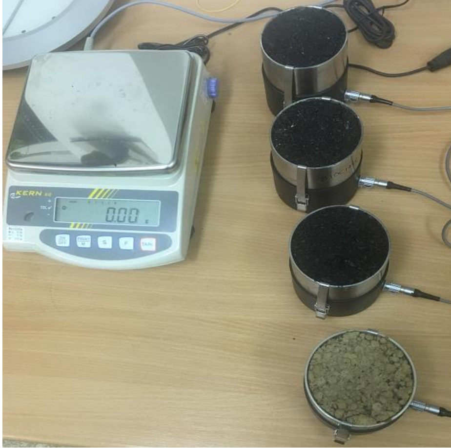
Figure 20. Samples are measuring with single balance mode (on the photo is one soil sample and three samples of pure biochar).
