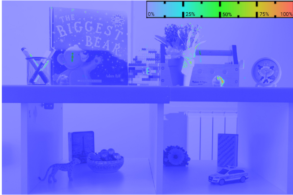
Figure 4.11: Figure shows „scene 1“ from Karaduzovic’s [16] dataset processed by the HDR-VDP2 [24] metric. The colour bar reflects the probability that an average observer will notice a difference between ghost-free HDR and ground truth HDR. De-ghosted HDR visual quality, according to HDR-VDP2 metric [24] is 73.24 (see Table 4.4).
