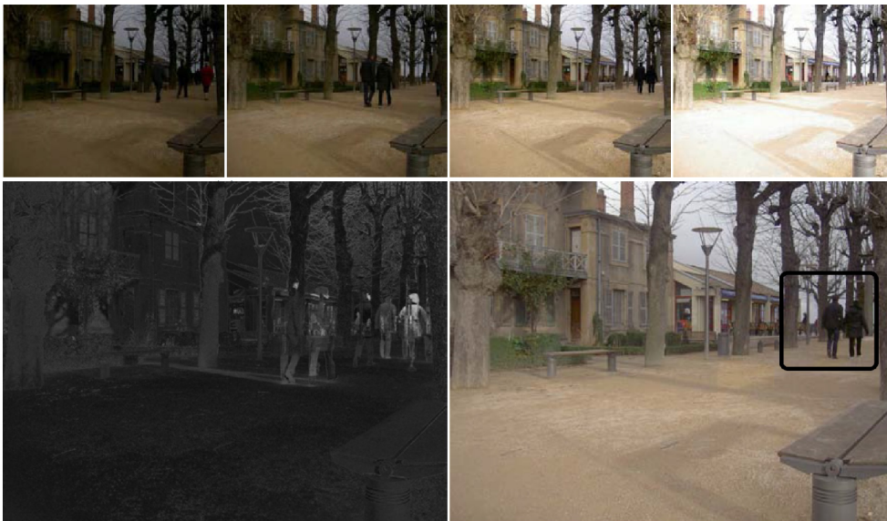
Figure 2.1: The Figure shows the results of variance based deghosting method by Jacobs et al. [12]. The variance map (bottom left) is obtained from the image sequence (upper row) and used to generate the HDR image (bottom right). Figure obtained from [12].
