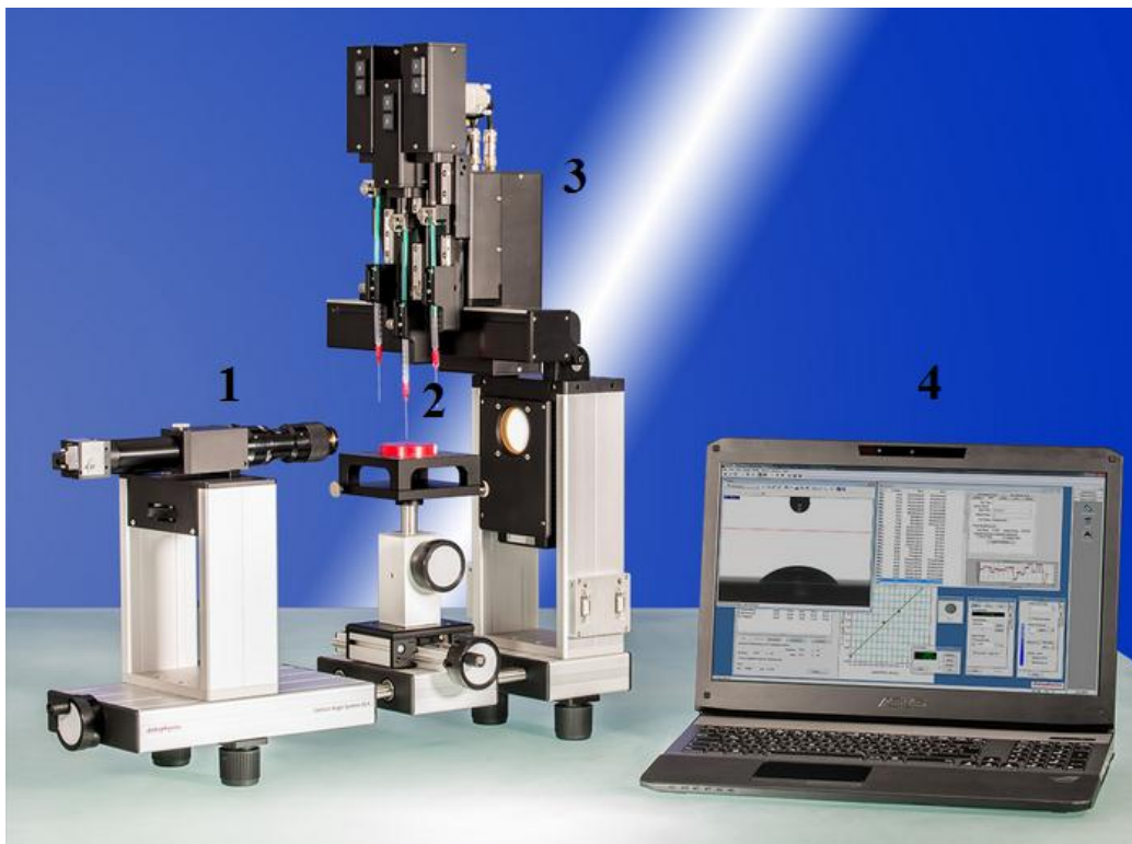
Fig. 14: The OCA 25 Contact angle measuring device [28]
