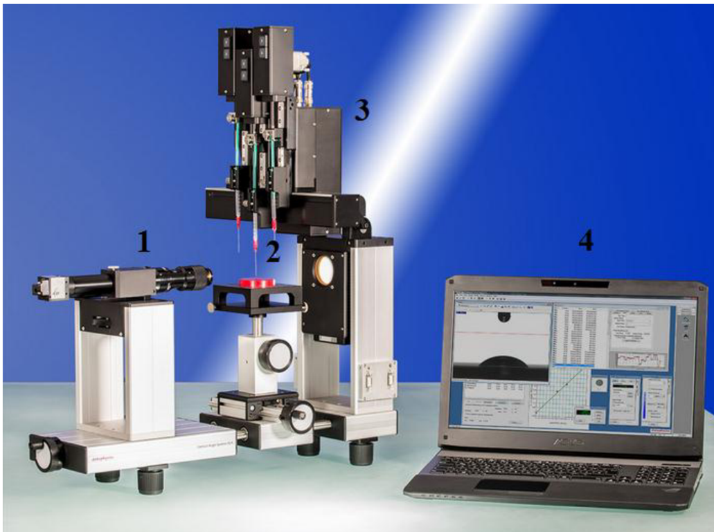
Fig. 14: The OCA 25 Contact angle measuring device [28]
