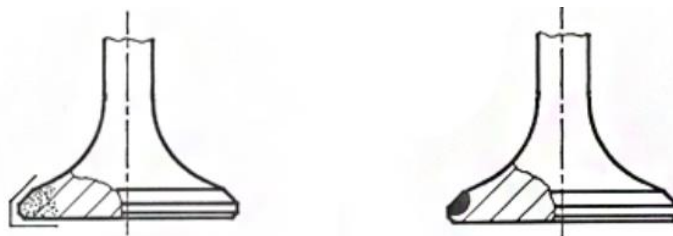
Fig. 6 Hardened valve head on the left side and hard facing on the valve head on the right side [1]
