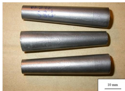
Fig. 46 Testing cones made from Stellite 6 and 12
