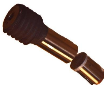
Fig. 36 Example of testing rod from material EN -GJS 450-8
