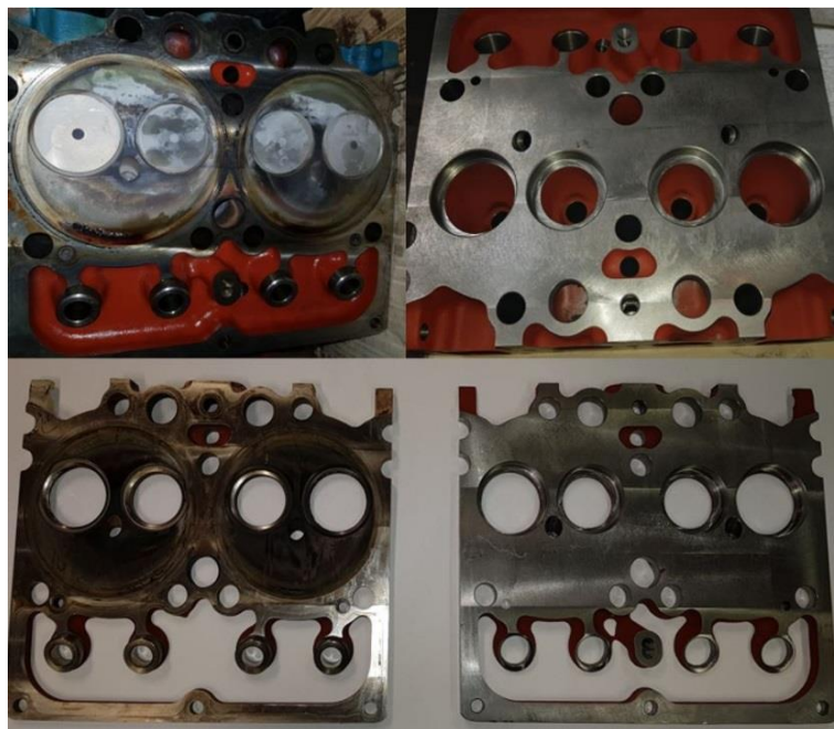
Fig. 104 Original cylinder head before and after preparing for testing
